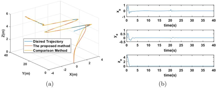
**Fig. 4.** Switched trajectory tracking: (a) Dynamic trajectory; (b) Position error
