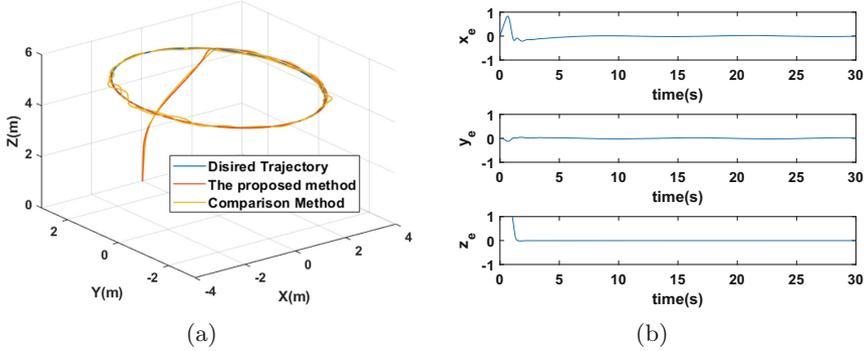
**Fig. 3.** Circular trajectory tracking: (a) Dynamic trajectory; (b) Position error
